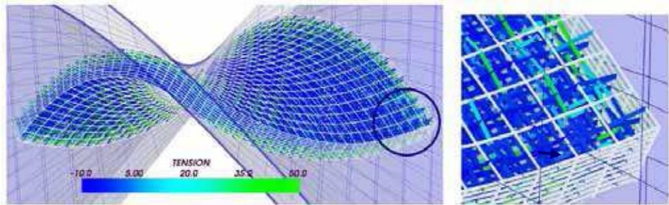
Fig. 24. Forming of a 3D interlock twisted plate
