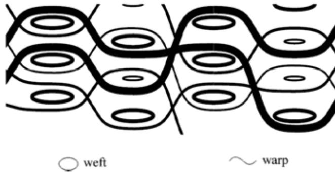
Fig. 22. Example of complex layer interlock weave
