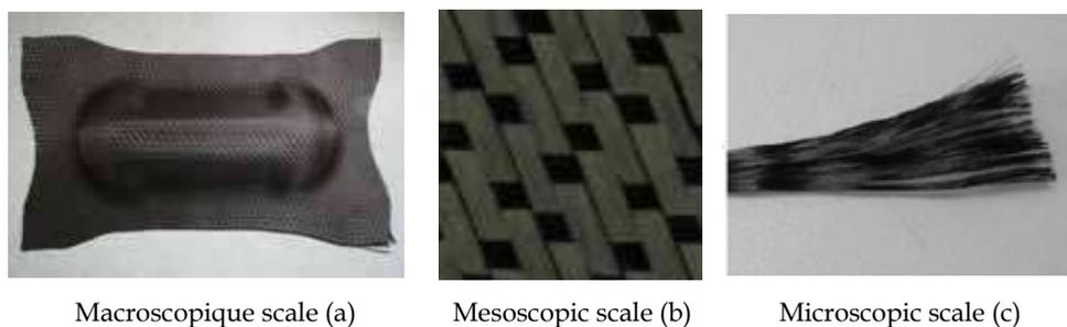
Fig. 5. The three scales of the fibre reinforcement
