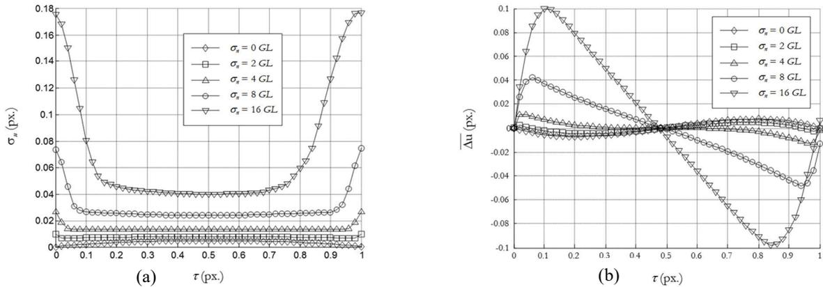
Figure 1.a – Evolution of the random error  $\sigma_u$  and 1.b – evolution of the bias error  $\overline{\Delta u}$  as a function of imposed displacement  $\tau$  for different noise levels  $\sigma_n$  for  $d = 16$  px.
