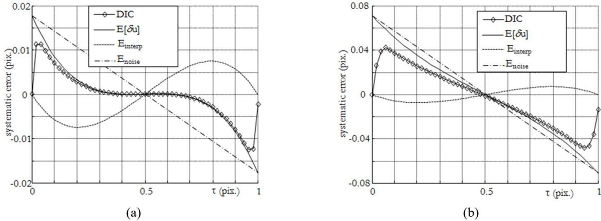
Figure 2 – Comparison of the experimental (DIC) and the theoretical ( $E[\delta u]$ ) bias errors as a function of imposed displacement  $\tau$  for  $\sigma_n = 4GL$  (Figure 2.a) and  $\sigma_n = 8GL$  (Figure 2.b)
