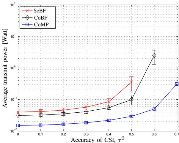
Fig. 5. Average transmit power in Watt vs.  $\tau^2$  when  $L = 16, K = 8, N = 32$  and  $r = 2$  [bps/Hz/UE].
