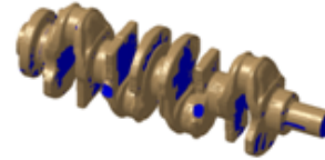
Figure 8: Crankshaft with scanning holes (in brown) and after hole filling (in blue).
