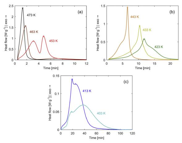
$\textbf{Fig. 3.} \ \ \text{DSC curves of isothermal syntheses of PA6, (a) for 453-463-473 \ K, (b) for 423-433-443 \ K \ and (c) for 403-413 \ K. \ and (c) for 403-413 \ K. \ and (d) for 403-413 \ K. \ and (d) for 403-413 \ K. \ and (d) for 403-413 \ K. \ and (e) for 403-$
