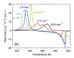
Fig. 1. DSC curves of non-isothermal syntheses of PA6 at different heating rates, (a) reactive mixture melting temperature range, (b) PA6 polymerization, crystallization and melting temperature range.
