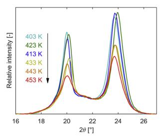
Fig. 8. WAXS scans of isothermally synthesized samples.
