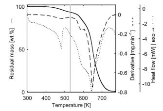
Fig. 7. TGA curve of a sample synthesized at  $2 \text{ K min}^{-1}$ .
