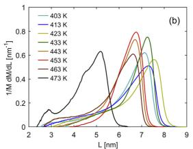
Fig. 9. Lamellar thickness distribution of PA6 crystalline phase, (a) for non-isothermal syntheses, (b) for isothermal syntheses.
