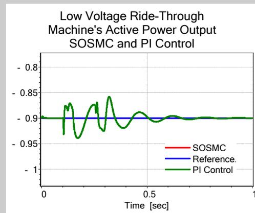
Fig. 4. Machine's Active Power Output after a short-circuit at the point of common coupling: comparison between Nonlinear (red) and Linear (dark green) Controller
