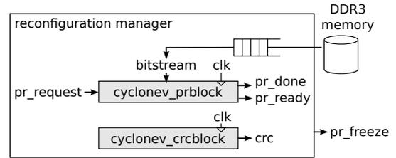
Fig. 5: DPR reconfiguration mechanism via DDR3 external memory
