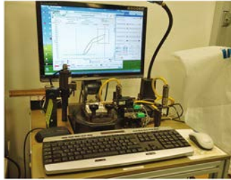
Fig. 6. Experimental test bench for contact/tripping force measurement.
