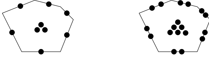
Figure 3: Uncut hexagonal cell. Left: k = 0 ; Right: k = 1 . Each dot attached to a geometric entity (face or cell) symbolizes one degree of freedom (not necessarily a pointwise evaluation).
