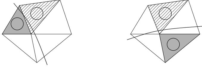
Figure 5: Triangular mesh cell  $T$  (filled by dashes) cut unfavorably by the interface; the companion cell in the agglomeration procedure is shown in gray for two generic situations: on the left, both cells share a face, and on the right, they only share a vertex; in both cases, the companion cell is in  $\Delta(T)$ , and the two balls in the agglomerated cell for Assumption 2 are shown.
