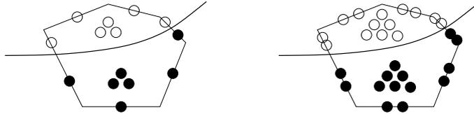
Figure 4: Cut hexagonal cell for the interface problem. The subdomain  $\Omega^1$  is located below  $\Gamma$  with the corresponding HHO unknowns shown by filled circles, and the subdomain  $\Omega^2$  is located above  $\Gamma$  with the corresponding HHO unknowns shown by empty circles. Left:  $k = 0$ ; Right:  $k = 1$ .
