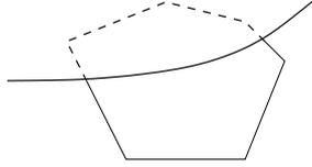
Figure 1: Hexagonal cell  $T$  cut by the interface  $\Gamma$ . The subdomain  $\Omega^1$  is located below  $\Gamma$ , and the subdomain  $\Omega^2$  is located above  $\Gamma$ .  $(\partial T)^1$  is shown using solid lines and  $(\partial T)^2$  using dashed lines; the sets  $\mathcal{F}_{(\partial T)^1}$  and  $\mathcal{F}_{(\partial T)^2}$  consist each of four elements, two of which are original faces of  $T$  and two of which are sub-faces of the two faces of  $T$  cut by the interface.
