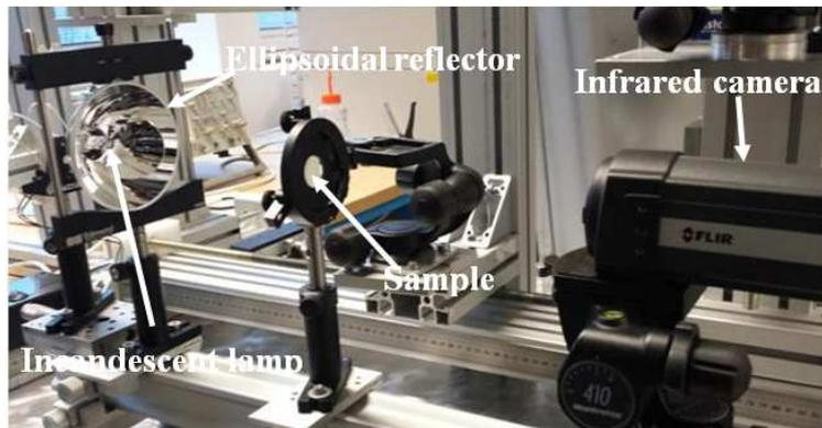
Figure 3: Experimental set-up
