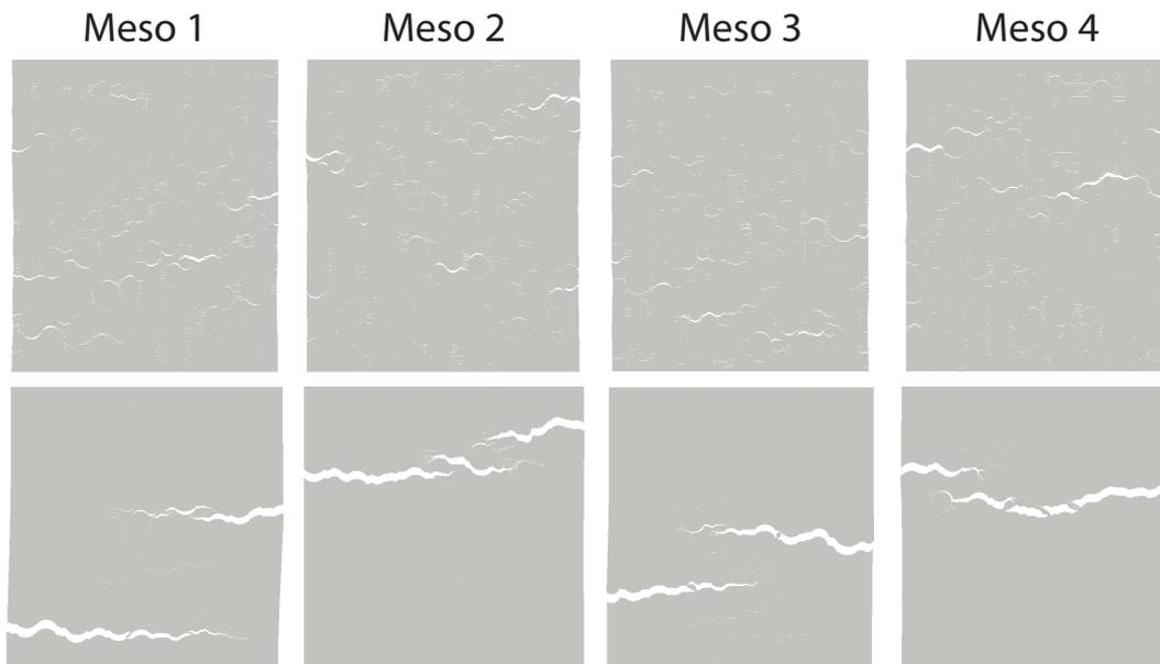
Figure 5: Influence of the meso-structure on the crack path for different meso-structures at  $\dot{\epsilon} = 0.1$  /s: upper row at  $\epsilon = 7.10^{-5}$  for  $\approx$  the peak stress (disp.  $\times 2000$ ), lower row at  $\epsilon = 3.10^{-4}$  (disp.  $\times 100$ )
