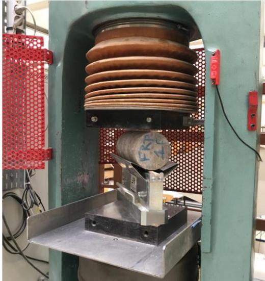
**Figure 2 : Settings of the splitting test**
