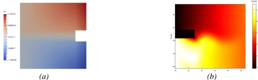
Figure 1. Displacement fields resulting (a) from the global FE analysis and (b) from experimental test using DIC [5].
