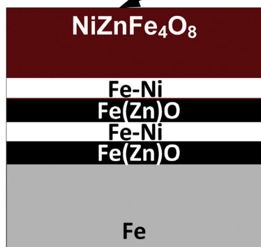
Fig. 10. Scheme of the reaction mechanism between iron and NiZn ferrite.
