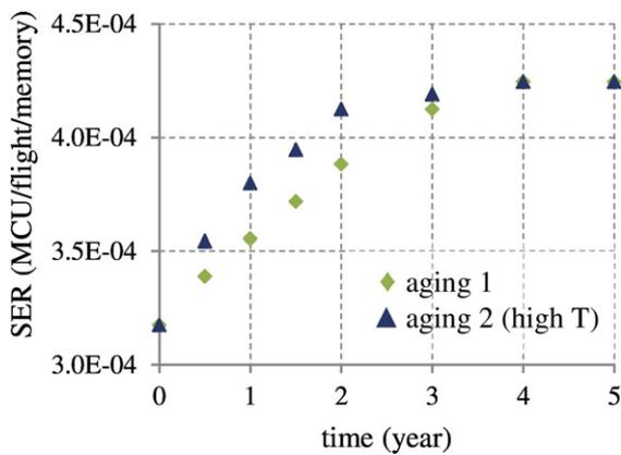
Fig. 7. Evolution of the SER over the lifetime of a 2 MB 6T SRAM bulk 32 nm for a Paris - New York flight.
