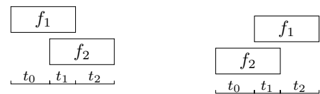
(a) A possible trace of execution for f_1 and f_2 (b) Another trace of execution
