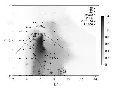
FIGURE 8. The wake patterns observed based on PIV data with approximate boundaries shown by the solid lines. This overlays a greyscale contour map of the mean peak amplitude, in  $U^*-\alpha$  parameter space, with amplitude levels indicated by the dashed lines. There appears to be a gradual change from 2P to P + S as the rotation is increased, causing a deflection of the wake away from the streamwise centreline.
