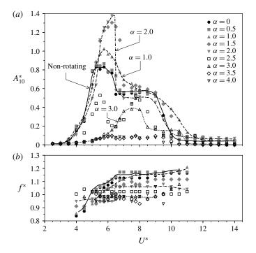
FIGURE 6. The vibration response of an elastically mounted circular cylinder undergoing constant rotation as a function of reduced velocity  $(U^*)$  at different rotation rates  $(\alpha)$ . (a) The normalised amplitude response  $(A_{10}^*)$ . (b) The normalised frequency response  $(f^*)$ . Approximate fits to cases  $\alpha = 0$ , 1.0, 2.0 and 3.0 are shown by the labelled dashed lines.
