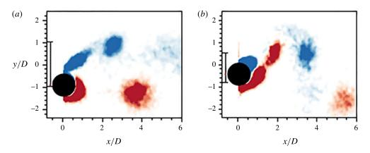
FIGURE 12. (Colour online) Phase-averaged isocontours of the P + S mode at  $U^* = 5.50$ ,  $\alpha = 1.15$  in the upper response branch (a) and  $U^* = 6.50$ ,  $\alpha = 0.60$  in the lower response branch (b). The normalised vorticity range is  $\omega^* = \omega D/U \in [-1, 1]$ .
