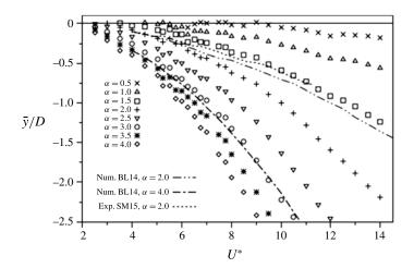
FIGURE 5. The time-averaged displacement of the cylinder  $(\bar{y})$  as a function of reduced velocity  $(U^*)$  at different rotation rates  $(\alpha)$ . Numerical predictions BL14 for Re = 100 at  $\alpha = 2.0$  and 4.0 are shown by the dot-dashed lines. The dotted line shows experimental results of SM15 at Re = 350-1000,  $\alpha = 2.0$  for comparison.
