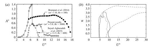
FIGURE 16. (a) Comparison of the response curve for  $\alpha = 2.0$  against previous numerical and experimental studies. Note, in particular, the much higher vibration response in this case. (b) Corresponding approximate vibration boundaries as a function of  $U^*$  and  $\alpha$ . Refer to panel (a) for data references.
