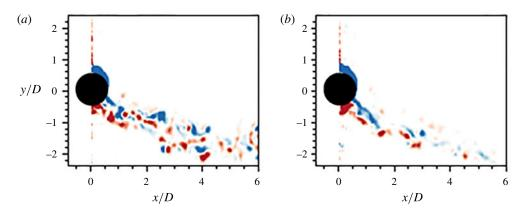
FIGURE 10. (Colour online) Instantaneous isocontours of the C(AS) mode at  $U^* = 4.00$ ,  $\alpha = 2.75$ . The C(AS) wake pattern is of a chaotic nature and consists of small vortices patched around a curve. The normalised vorticity range is  $\omega^* = \omega D/U \in [-1, 1]$ .
