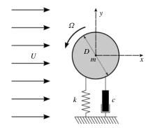
FIGURE 1. Definition sketch for the transverse FIV of a rotating cylinder. The hydroelastic system is simplified as a 1-DOF system constrained to move in the cross-flow direction. The axis of rotation is transverse to both the flow direction (x-axis) and the oscillation axis (y-axis). Here, U is the free-stream velocity, k the spring constant, D the cylinder diameter, m the oscillating mass, c the structural damping and  $\Omega$  the angular velocity.
