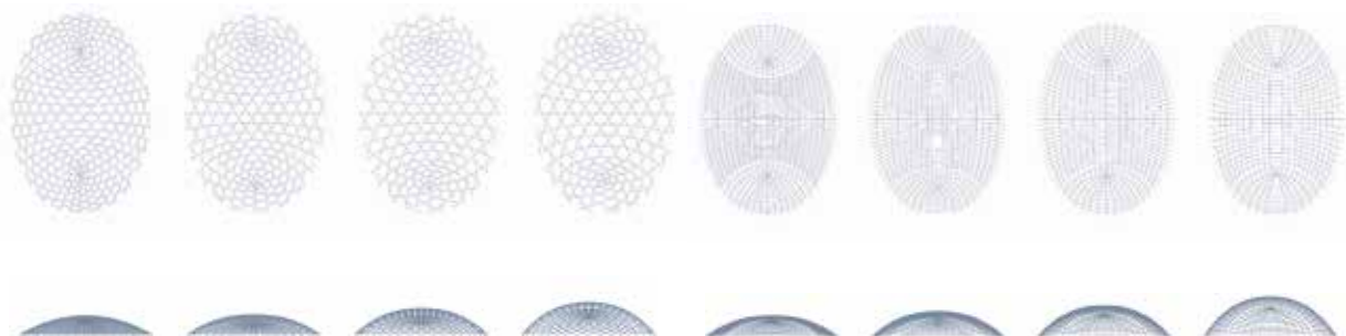
Figure 13: Several optima in the Marionette Design space: shallow structures are heavier and feature more nodes, the Kagome grid pattern yields better results for our performance metrics
