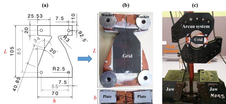
Figure 1: dimensions of specimen (a), Wood specimen (b); experimental device (c)
