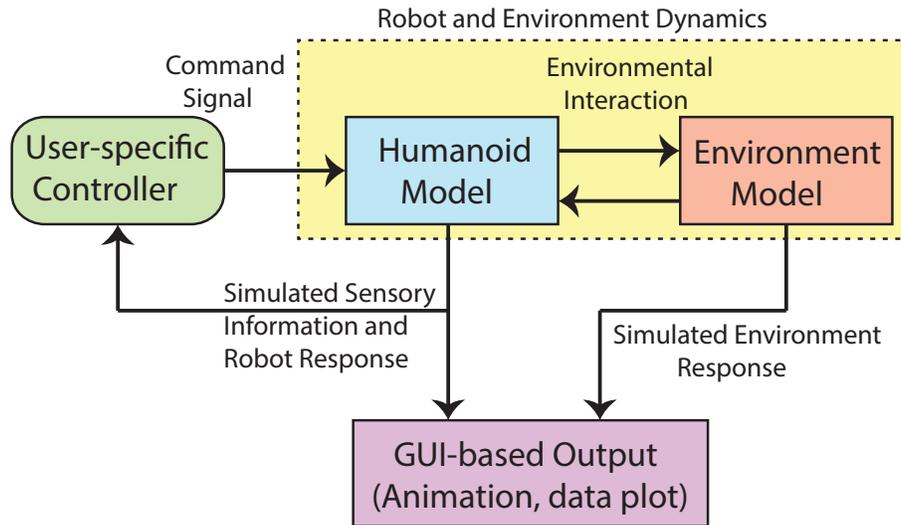
**Fig. 1** Fundamental elements of a humanoid robot simulator.
