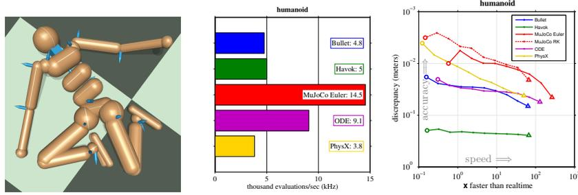
**Fig. 9** Image courtesy of Tom Erez, Yuval Tassa and Emanuel Todorov [50]. The first image illustrates the simulated humanoid. The second image shows raw speed as thousands of evaluations per second for each engine. The third image shows the speed-accuracy trade-off in terms of our consistency measure.
