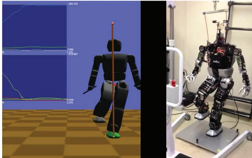
**Fig. 6** The humanoid robot Hubo is one of the template models in K'lamp [26]. In this study, both the simulated robot and actual robot simultaneously perform balancing on a single leg. The accuracy of the simulator is verified by comparing the actual sensory data and simulated sensory data. Image courtesy of Kris Hauser.
