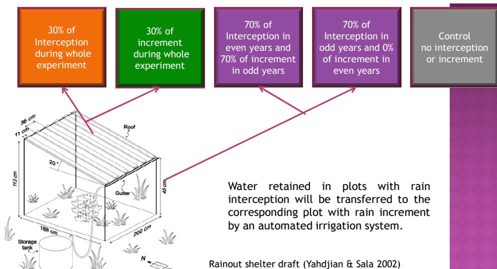
The rainfall increment treatment, rainfall intercepted by the shelters is diverted to a temporary tank and then pumped to the irrigated plots.
