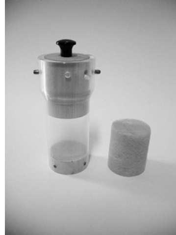
Figure 7. Compression device: (a) general scheme; the bottom extremity is fixed to the tube and the top extremity slides vertically between two pre-selected positions, (b) photograph showing the device and the sample.
