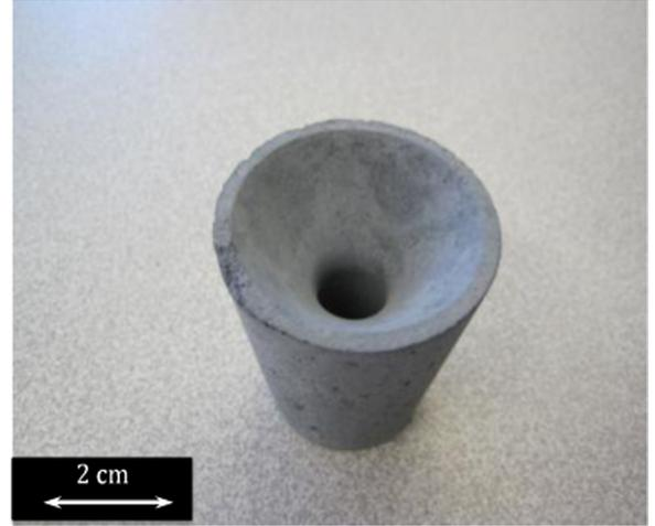
Fig. 2. SiC-based micro-concrete nozzle after manufacturing.
