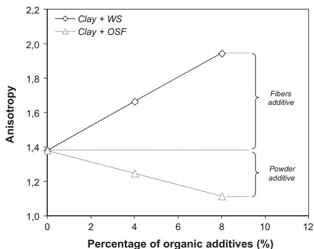
**Fig. 5.** Anisotropy of the clay ceramic and of the clay ceramic with a 4 wt% and an 8 wt% addition of OSF and WS after a firing process at 900 °C.
