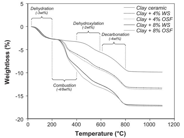
Fig. 2. Thermal behavior of the clay ceramic and of the clay ceramic with a 4 wt% and an 8 wt% addition of OSF and WS.
