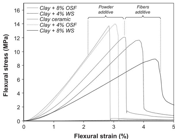
**Fig. 7.** Flexural stress-strain curves of the clay ceramic and of the clay ceramic with a 4 wt% and an 8 wt% addition of OSF and WS after a firing process at 900 °C.
