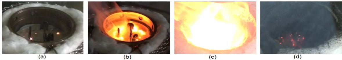
Figure 4: The progress of Chris(X)ti-Na experiment (a) sodium oxide crust with some apparent nodules, (b) the propagation of the nodules, (c) sodium combustion established, and (d) the beginning of sodium fire's extinction with the extinguishing powder.
