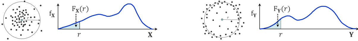
Fig. 1: The random distance variables \mathbf{X} and \mathbf{Y} have different LID values at distance r . Although the total probability measures within distance r are the same (that is, F_X(r) = F_Y(r) ), ID_{F_Y}(r) is greater than one would expect for a locally uniform distribution of points in \mathbb{R}^2 , while ID_{F_X}(r) is less.
