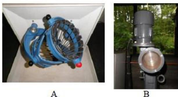
**Fig. 1.** Experimental set-up for iron ore granulation: picture (A) shows the turbula shaker-mixer used for homogenisation procedure while picture (B) illustrates the drum granulator used to create granules.
