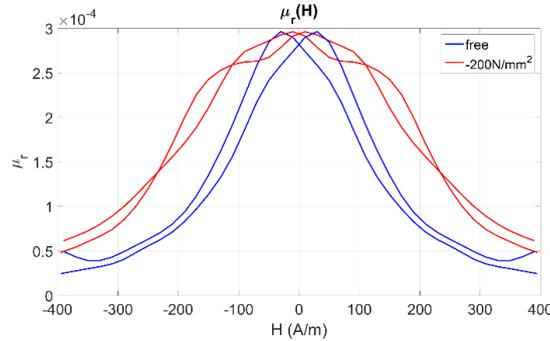
Fig. 1 – Evolution of the RMS permeability versus the excitation field  $H$  for a free sample and a stressed one.
