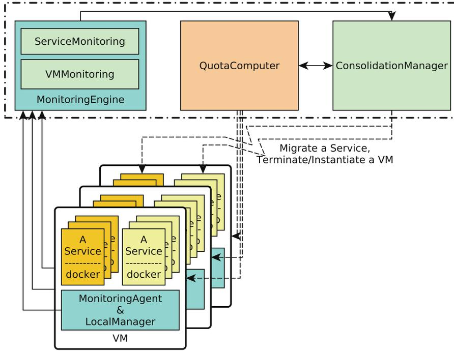
Fig. 1. Architecture of our software consolidation system
