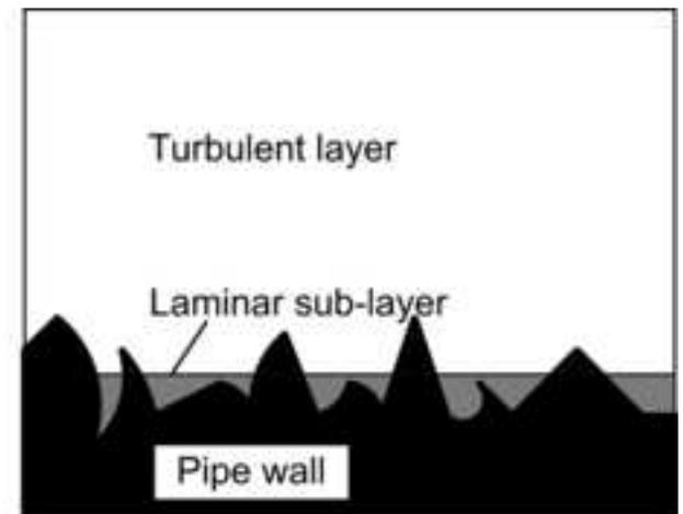
c) Hydraulically rough pipe
