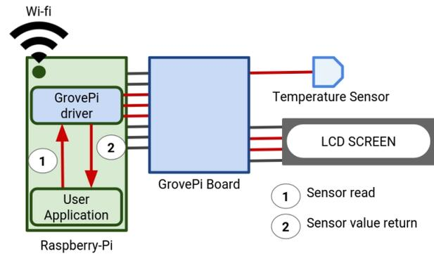
**Figure 1.** CPS scenario. A Raspberry Pi with a GrovePi board controls LEDs, a temperature sensor and an LCD screen. The developer remotely deploys, tests and interacts with the application from his development machine through WiFi.
