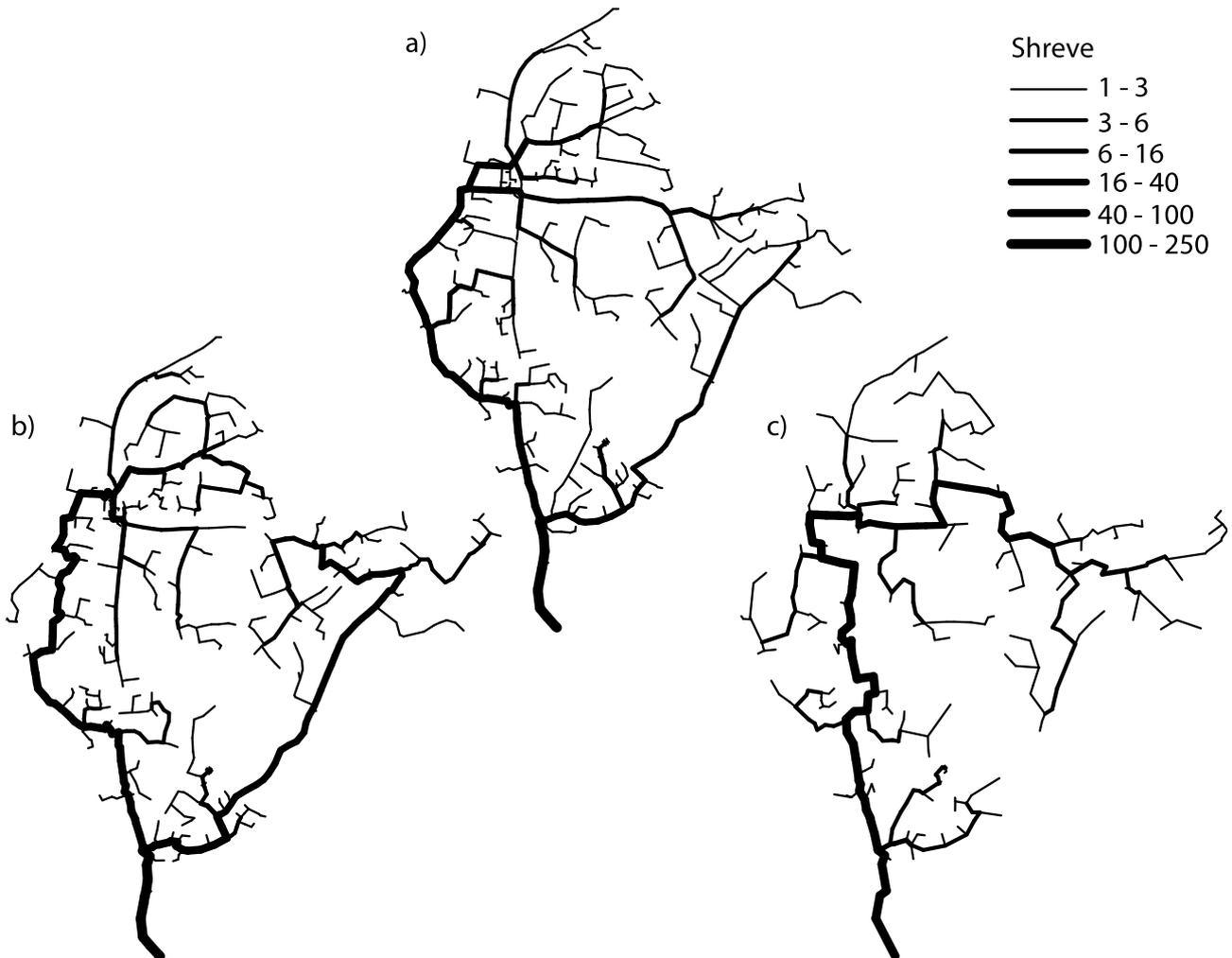
*Fig. 1 Comparison between the actual and reconstructed networks using cost function 1 and  $\alpha=0.9$ ,  $\beta=2$  and  $\gamma=5$ . a) The actual network; b) The reconstructed network using the entire dataset; c) The reconstructed network using half of the manhole cover locations.*
