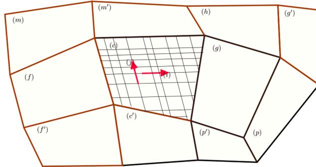
Fig. 1: Surface of the large-network (as the network-domain) is dis-aggregated in  $2d$ -zones. Zones are meshed in quadrangular cells. Each cell has certain parameters: a finite number of preferred propagation directions of flows, numbers of lanes in each direction, lengths of lanes in each direction.
