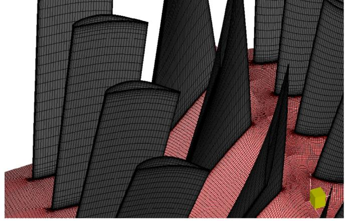
Fig. 2. 3D view of the stage indicating mesh.
