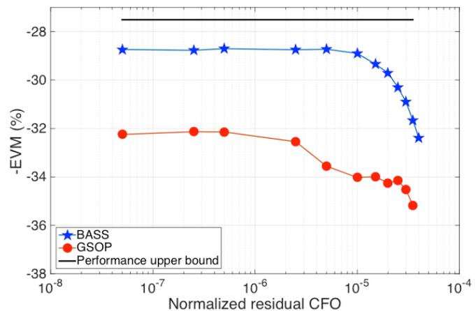
Fig. 6. Average EVM as a function of the normalized residual CFO with 4-QAM modulations. The sets of gain/ phase imbalance values of polarizations X and Y are 1.2/  $30^\circ$  and 1.1/  $30^\circ$ , respectively.
