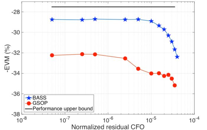
Fig. 6. Average EVM as a function of the normalized residual CFO with 4-QAM modulations. The sets of gain/ phase imbalance values of polarizations X and Y are 1.2/  $30^\circ$  and 1.1/  $30^\circ$ , respectively.
