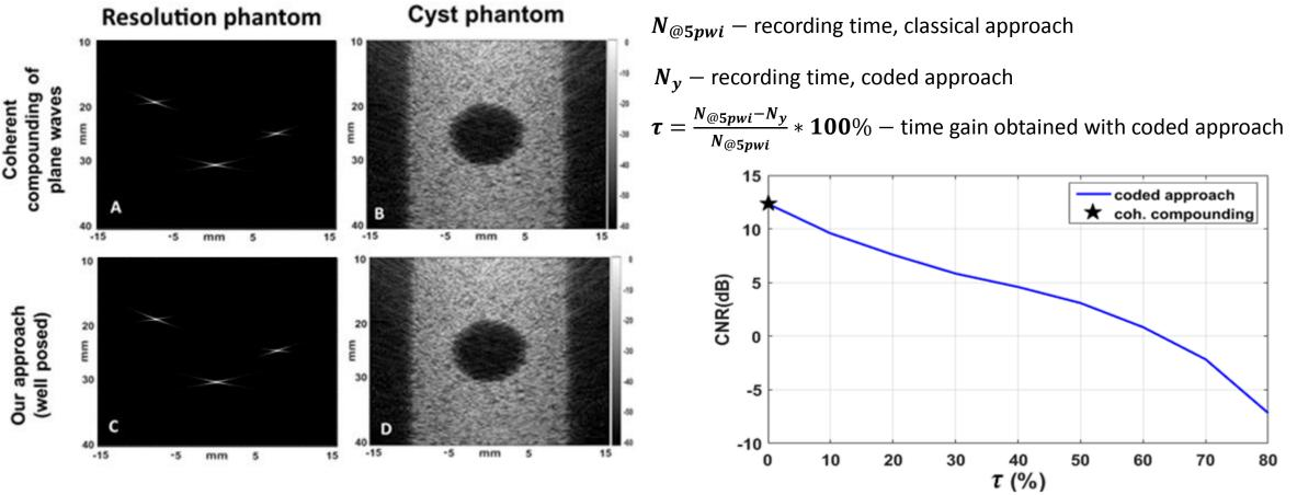
Reducing the observation time adds a Perturbation Zone, that makes the system ill-posed thus the CNR drops
