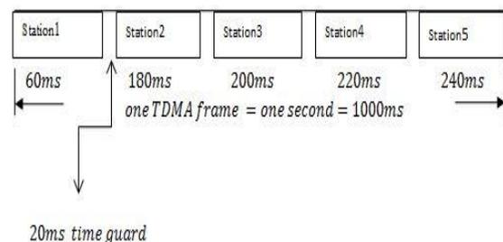
Figure 6: shows the TDMA frame and time slot allocated for video and audio bitrate for VSAT stations.
