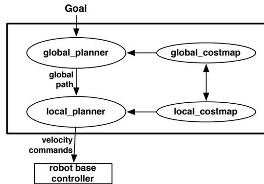
Fig. 1: Concept of navigation methods ([www.ros.org/wiki/move\\_base](http://www.ros.org/wiki/move_base))
