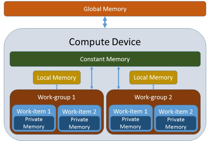
Fig. 2. Intel FPGA SDK for OpenCL Memory architecture.
