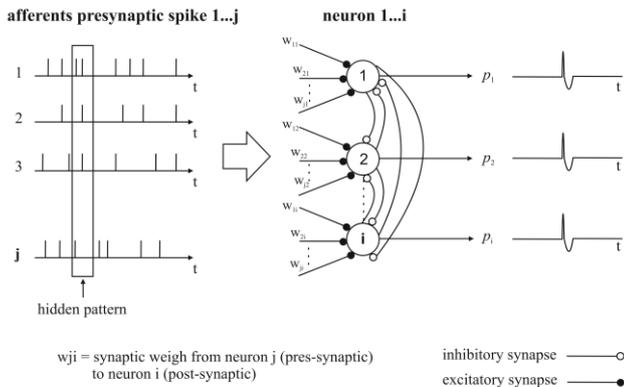
**Fig. 1.** Architecture of a neuronal network listening incoming spike trains with hidden patterns
