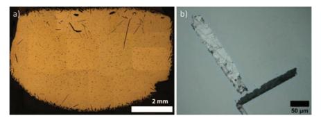
**Fig. 5.** a) Photomontage of light micrographs showing a sample of flake graphite iron produced by remelting the initial spheroidal graphite alloy and b) polarized light micrograph of graphite flakes. (A color version of this figure can be viewed online.)
