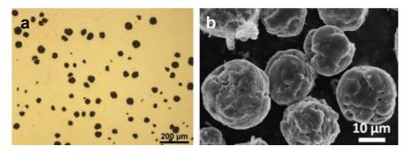
Fig. 1. a) Optical micrograph of a spheroidal graphite cast iron section and b) SEM image of extracted spheroids. (A color version of this figure can be viewed online.)
