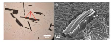
Fig. 8. a) Optical micrograph of typical flakes obtained in Fe-C alloy, b) SEM image of a flake after deep etching. (A color version of this figure can be viewed online.)
