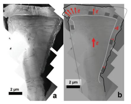
**Fig. 13.** a) Photomontage of bright field TEM images of a sector of primary exploded graphite b) schematic of graphene stacks with the *c* axis orientation indicated by arrows. (A color version of this figure can be viewed online.)
