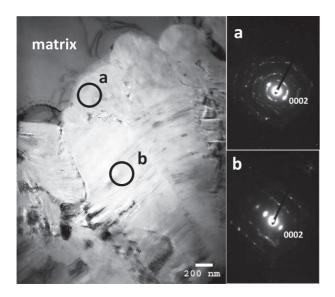
**Fig. 2.** Bright field TEM image of a sector in a graphite spheroid combined with SAED patterns a) at the periphery and b) in the bulk of the sector (the selected areas used to perform diffraction are schematized by the two black circles in the bright field image).
