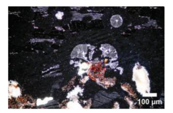
**Fig. 12.** Optical dark field micrograph of a Fe–C–Ce alloy – Graphite: grey, matrix: black, Ce and O: red and porosity: white. (A color version of this figure can be viewed online.)
