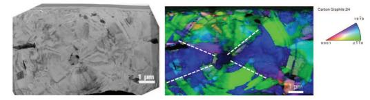
**Fig. 3.** Photomontage of TEM images of a diametrical section of graphite spheroid combined with the crystal orientation map of graphite obtained by ACOM; apparent boundaries between sectors are highlighted by white dotted lines (dark areas at the periphery of the nodule are iron-rich particles that were not indexed). (A color version of this figure can be viewed online.)
