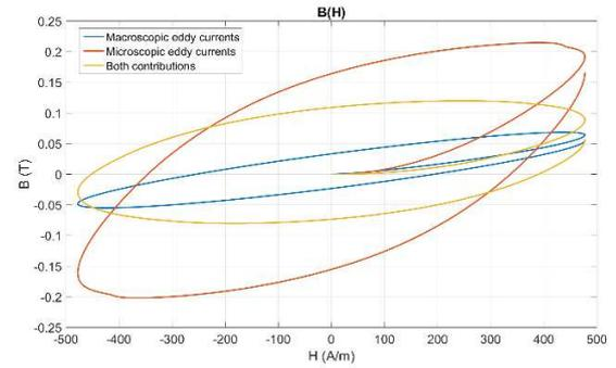
Fig. 1. Hysteresis loop considering different losses contribution.
