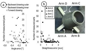
**Figure 10.** Geometry measurements of 75 representative SSF forged parts: a) Error of the extrusion angles and b) straightness error of the four laterally-extruded arms.
