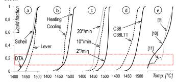
**Figure 1.** The experimental determination of liquid fraction as a function of temperature is influenced by a) the experimental / calculation method (DTA = Differential Thermal Analysis), b) reheating vs cooling method, c) the heating rate. d) Differences between regular vs thixoforging-specific metallurgical variants of a steel grade are of the same order of magnitude as the previous effects, or as the differences between measurements by different labs (e) [9]-[11].
