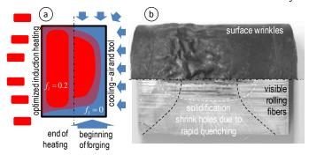
**Figure 2.** a) Principle of temperature gradient creation during induction heating and transfer to press and b) its trace observed on reference billets quenched after a heating-transfer cycle to reveal the temperature and metallurgical state before SSF: the colder ends preserve traces of fibering and the original outer geometry, while the central zone exhibits the signs of high liquid fraction: solidification shrink holes at core and surface wrinkles at the surface.
