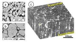
**Figure 4.** A posteriori liquid fraction determination by various methods on M2 steel: a) optical microscopy (after quenching), b) confocal laser scanning microscopy and c) 3D reconstruction of liquid zone and solid skeleton by X-ray tomography [16].
