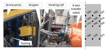
**Figure 3.** Robotized cell and induction heating furnace with controlled atmosphere at LCFC (left) and measured temperature field (in °C) at the end of induction heating (right).
