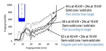
**Figure 7.** Force-stroke plots for one part geometry and three different part heating cycles.
