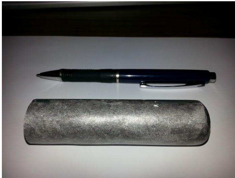
Figure 1: Typical Fe-Al-B alloy bar of 25 mm in diameter and 110 mm in length
