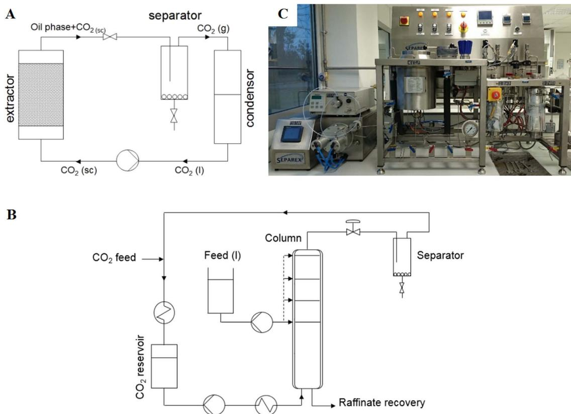
Fig. 4. Simplified schematic representation of supercritical CO<sub>2</sub> installation for solid extraction (A) and liquid extraction (B), example of supercritical fluid lab scale equipment – 1 L autoclave (C).
