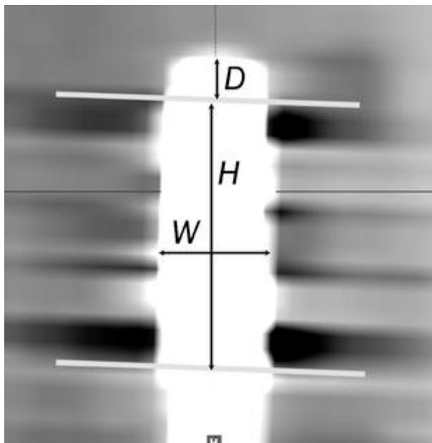
*Figure 3. Illustration of the different artefact parameters measured on phantom and patient CT acquisitions.  $W$  maximal width of the white electrode artefact,  $H$  height of lateral black artefact along the electrode axis,  $D$  distance between the beginning of the white electrode artefact and the beginning of the lateral black artefact.*
