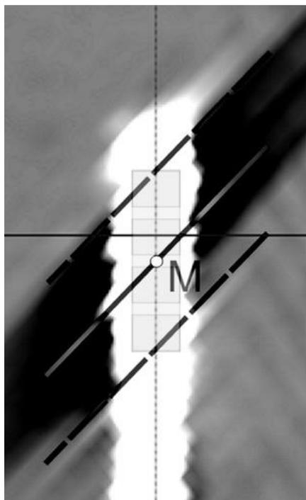
*Figure 7. After identification of the distal and proximal black artefact boundaries (dotted lines), the location of the four contacts is determined relatively to the point ( $M$ ) placed in the middle of the distance between the two boundaries.*
