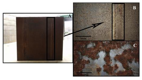
Fig. 1. A) Plow sculpture photograph. B) Detail of the steel part in contact with the wooden pallet. C) Detachment process detail.
