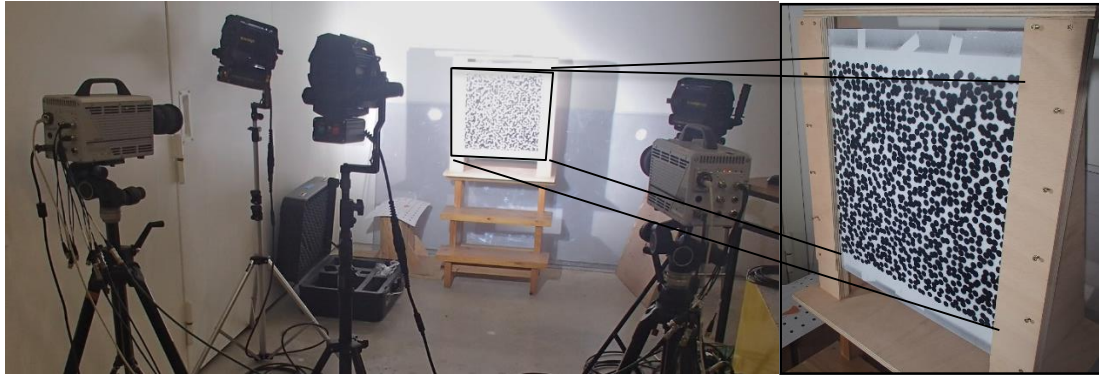
Figure 1. Stereo-correlation device comprising high speed camera and large scale target with coarse speckle pattern.
